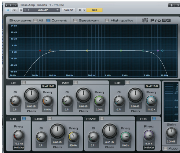
FIG. 3: PreSonus' ProEQ plug-in for Studio One provides five fully parametric bands of EQ plus a high-cut filter and a low-cut filter. The low- and high-frequency bands (LF and HF) are shelving filters.
