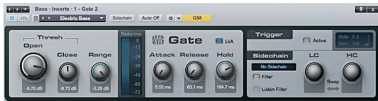
FIG. 4: Gating a vocal with Studio One's Gate plug-in. Since vocals are slow-rising signals, in terms of dynamics, we're using a slow attack time.
