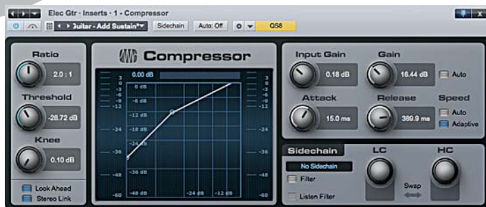
FIG. 2: The term “knee” refers to the way the compression curve bends at the threshold point when represented. This curve shows hard-knee compression.
