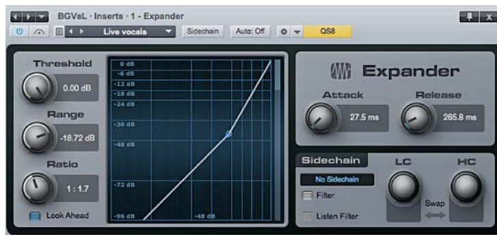
FIG. 3: This full-featured Expander plug-in includes a sidechain with Key Filter and Key Listen.
